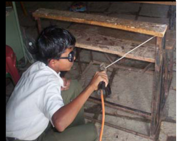
Applying welding skills to repair a classroom bench
